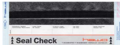
1. Intact seal for a specified seal width in accordance with ISO 11607, Part 2
